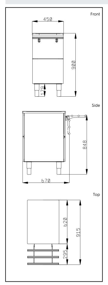
$\qquad \qquad \text{Flexy Compact} \\ \text{Ambient Unit on cupboard (1 GN) with one stainless steel tray slider}$
